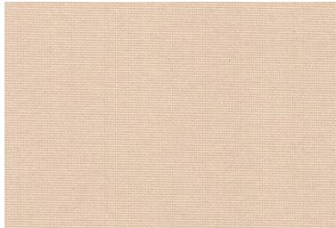
FIBERLUXE Architectural Membranes are designed for use as permanent tensioned membranes. These membranes feature a tightly woven fiberglass fabric coated with PTFE - FIBERLUXE Membranes allow diffuse natural light in while providing the strength needed for long spans in lightweight construction.
