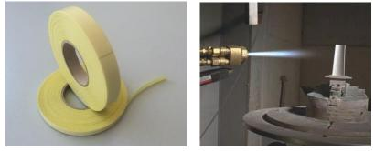
The automotive and aerospace industries some mechanical parts are highly loaded with temperatures, corrosion and erosion. To protect them against these heavy influences, plasma spraying is the solution.
